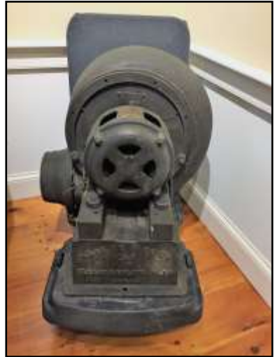
Hydrogen pump used to inflate blimps at the Chatham Naval Air Station during WWI.
